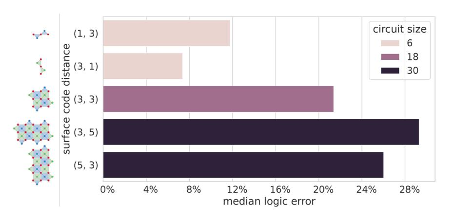
**XXZZ code results.** Top: logical error (vertical axis), i.e. the chance for the surface code to fail given the radiation fault's time evolution and noise intensity. Bottom: how the code's distance, i.e. the number of time the information is replicated, affects the logical error.
