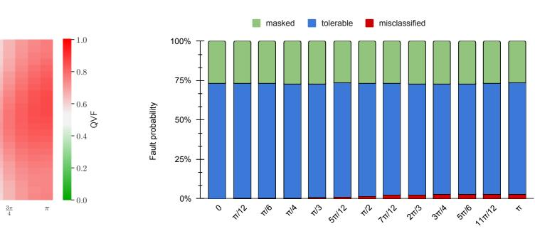
Quantum layer response to logical errors. Quantum Vulnerability Factor for single logical-shift fault injections.
