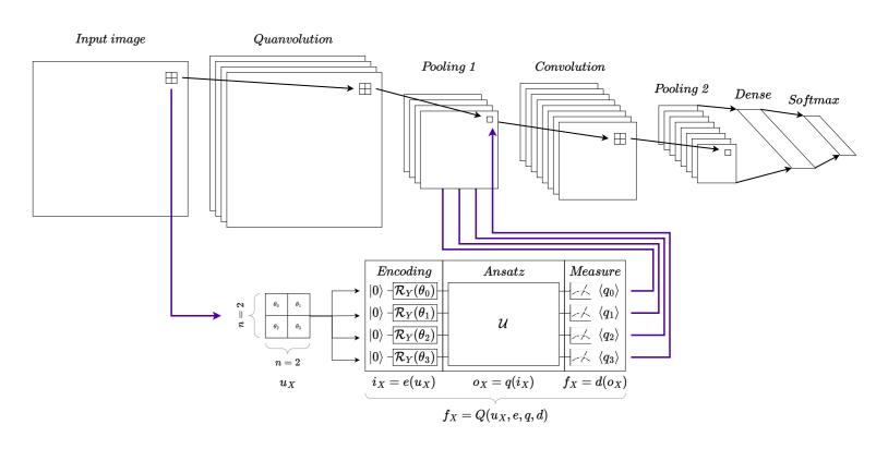
Quanvolutional neural network. In this hybrid model, a quantum convolutional layer feeds into other classical layers to perform image classification.
