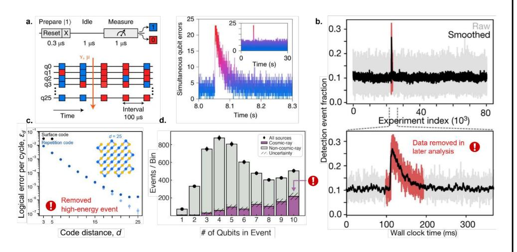
Experimental evidence. Many recent papers highlighted radiation induced correlated multi-qubit errors. a. McEwen et al., 2022. b. Chen et al., 2021. c. Acharya et al., 2023. **d.** Harrington et al., 2024.
