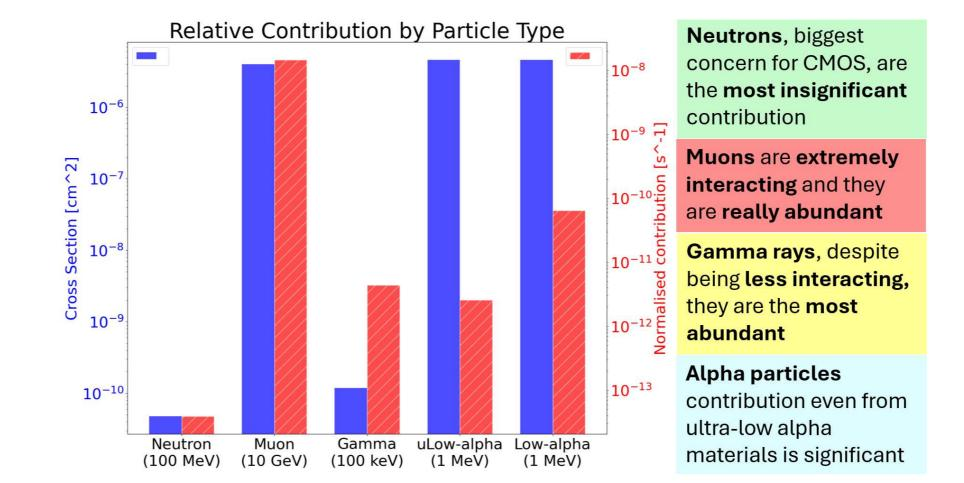
Different particles contribution. The left axis shows the cross-section (blue) and the right one is the cross-section multiplied by the flux of that particle at sea level (red).
